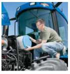
grill swings open for easy access to the radiator and cooling system. A radiator overflow bottle allows for quick visual checks of
